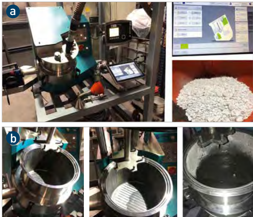
The single-chamber reactor pilot plant, developed and constructed to produce welding powder for aluminum submerged arc welding: a) The overall pilot plant in operation, b) The pilot plant shortly after a dummy run carried out for evaluation purposes
