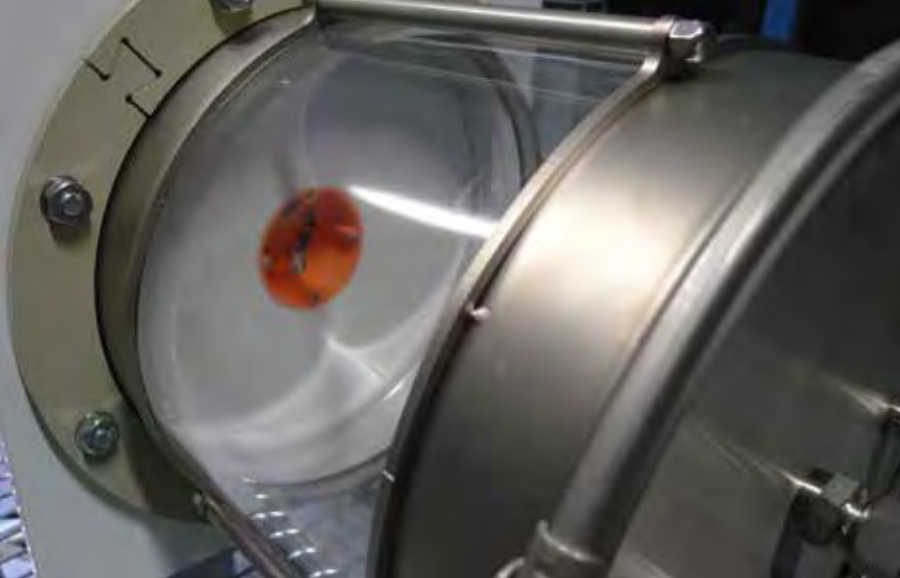
↑ Test rig for conducting quantitative assessments on the airtightness
